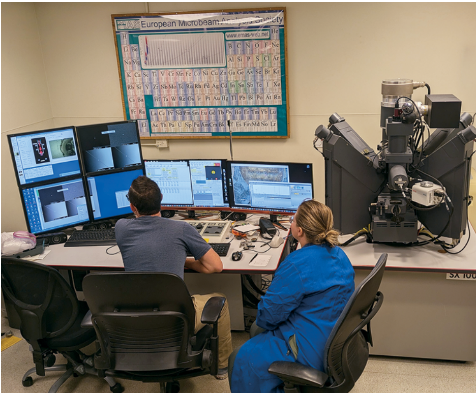
Student and staff operating the Electron Probe Micro Analyser (EPMA) in the Electron Microscopy facility to acquire chemical compositions and map the distribution of elements across microscopic areas of a rock sample. Photo: Lee Sharpnack
